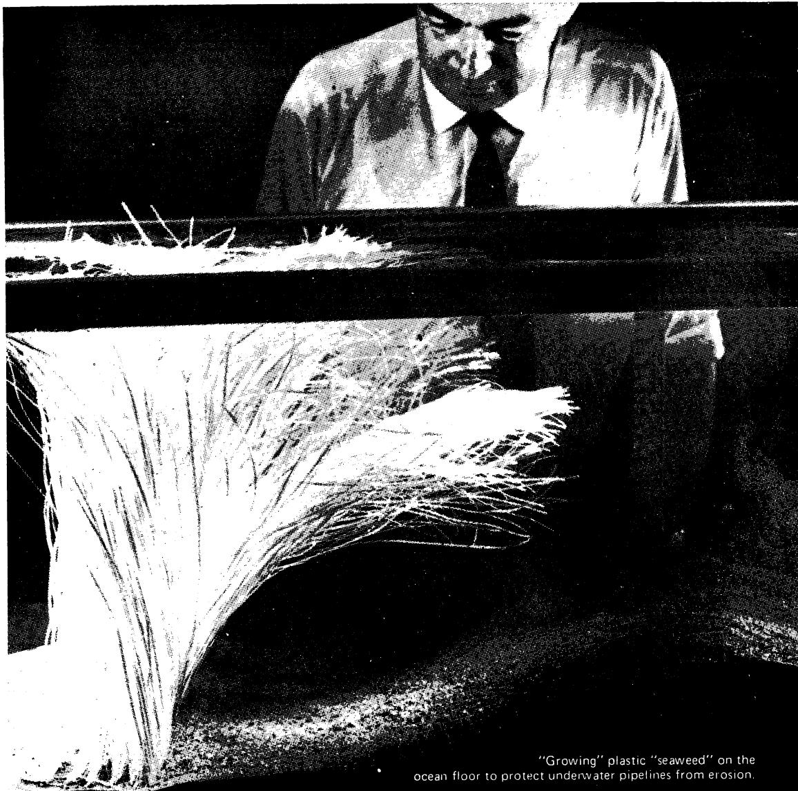
"Growing" plastic "seaweed" on the ocean floor to protect underwater pipelines from erosion.
